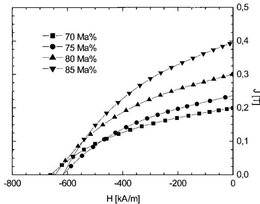
Figure 2 Demagnetization curves at room temperature of cured MQP-B inks with various loading of magnetic powder.
