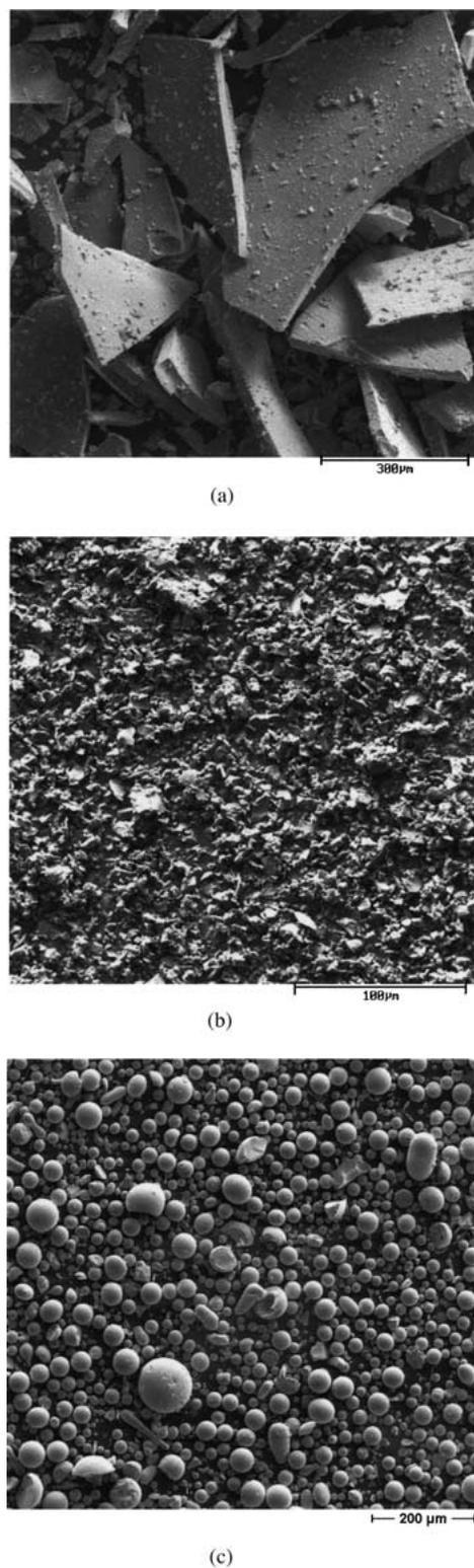
Figure 1 REM micrograph of powders MQP-B, original flakes (a) and powder milled for 24 h (b) and MQP-S original spherical powder (c).
