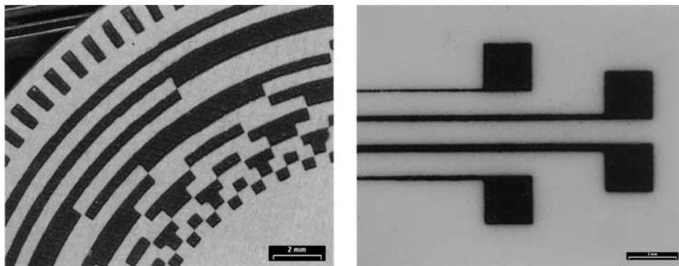
Figure 7 Micrographs of screen printed MQP-B films on an iron (left) and ceramic (right) substrates for sensor applications.
