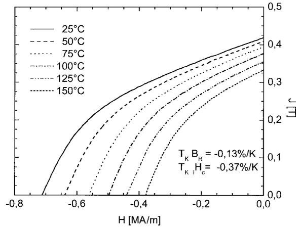
Figure 4 Demagnetization curves of a cured MQP-S ink (91 wt%) at different temperatures.
