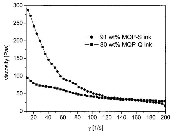
Figure 5 Room temperature viscosity as a function of shear rate of inks with 80 wt% of MQP-Q and 91 wt% of MQP-S.
