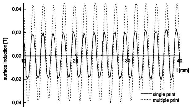
Figure 6 Induction across the surface of a printed MQP-B film magnetized with 1 mm pole pitch (measured  $250 \mu\text{m}$  above the surface): single print with about  $10 \mu\text{m}$  film thickness (solid line) and multiple print with about  $50 \mu\text{m}$  film thickness (dotted line).
