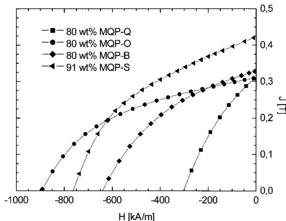
Figure 3 Demagnetization curves at room temperature of MQP-B, MQP-Q, MQP-O inks (80 wt%) and MQP-S ink (91 wt%).
